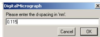
In this calibration, the user should use the microscope kV value together with measured first ring size (in pixels) to work out the relationship of diffraction angle/pixel, i.e. mrad/pixel. If the kV value is incorrect, the calibration is in error. This will affect the subsequent beam tilt calibration and hence the overall accuracy of the tuning procedures
