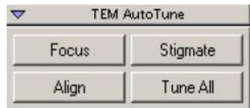
A good autotuning start-point is that the TEM should be roughly at the correct pre-alignment condition. The auto tuning is not effective when the TEM is severely mis-aligned.
