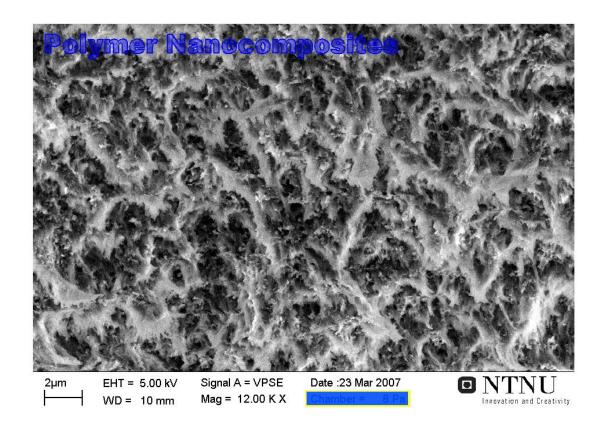
The VPESEM image demonstrated clearly the nano-particles in the polymer.
