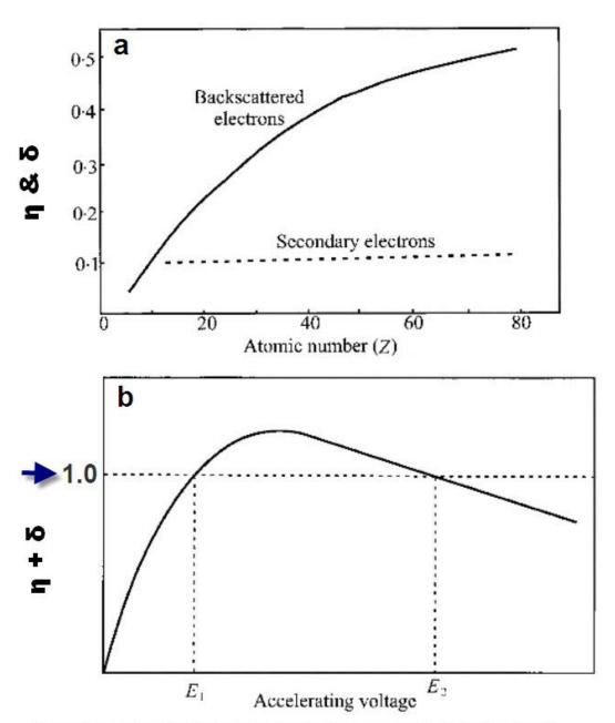
As we learned early, the backscattered electron coefficient  $\eta$  is strongly dependent on the atomic number of the specimen but the secondary electron coefficient  $\delta$  is not as shown in Figure (a). The total electron yield is a complex function of accelerating voltage, with a maximum between the crossover points E1 and E2 (around 1-5 keV) as shown in Figure (B). As  $\eta$  is almost independent of voltage, Figure (b) effectively represents the voltage dependence of  $\delta$ .
