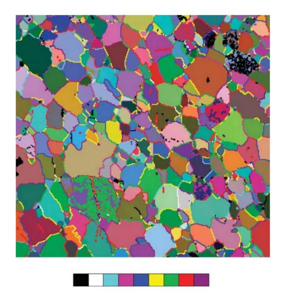
Orientation map of calcite grains in marble derived from EBSD patterns; misorientations across boundaries colored according to scale shown (0-90 degree).
