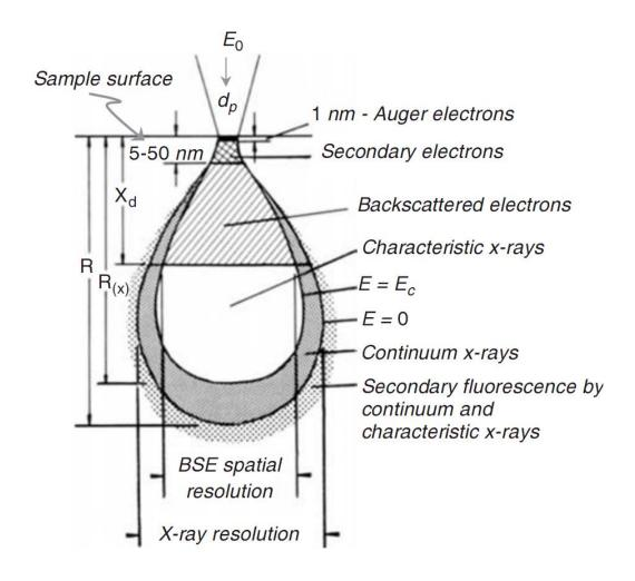
Schematic diagram to show the interaction volume of the primary electron beam.
