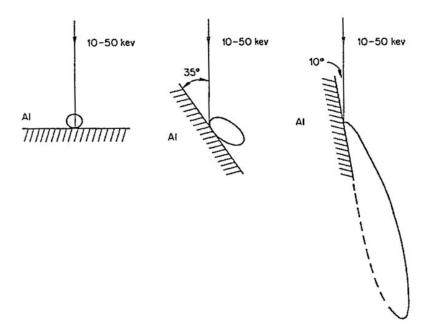
Since BSE has relative higher energy, it is not so easy to be deflected! Therefore it is very important to have a correct BSD detector setting, which is totally different as that for Normal beam incidence).... see later EBSD discussion.
