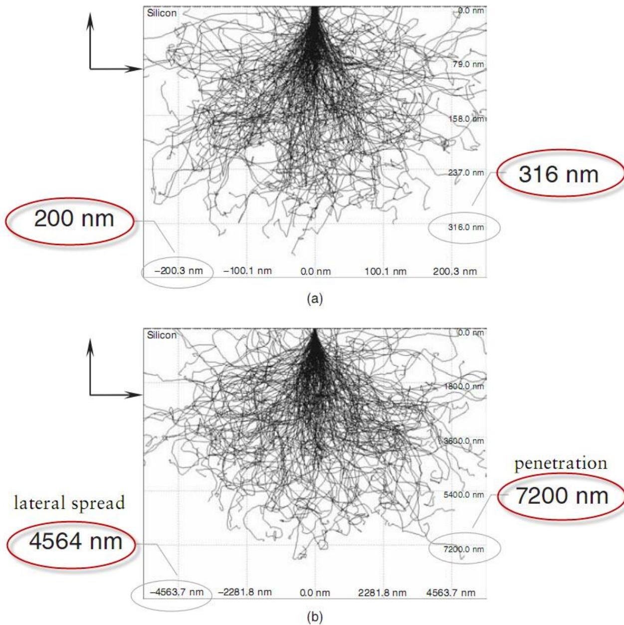
The interaction volumes for low vs high primary electron energy  $E_0$  in a silicon substrate ( $Z = 14$ ). (a)  $E_0 = 5 \text{ keV}$ ; (b)  $E_0 = 30 \text{ keV}$ . The lateral spread and penetration depth are much increased in the case of (b).
