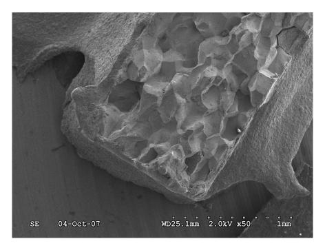
For further finding the reason of intergranular fracture, happened due to precipitate free zones around GBs in this material, we have to carry out TEM investigation during TEM Lab in week 14.
