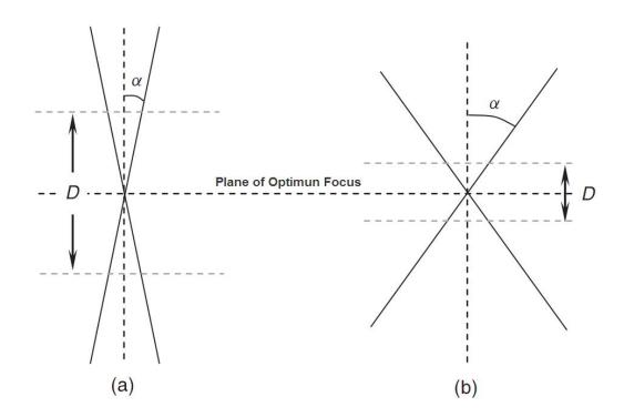
The large and small values of  $\alpha$  (divergence or convergence semi-angle) and the effect on the depth of field.
