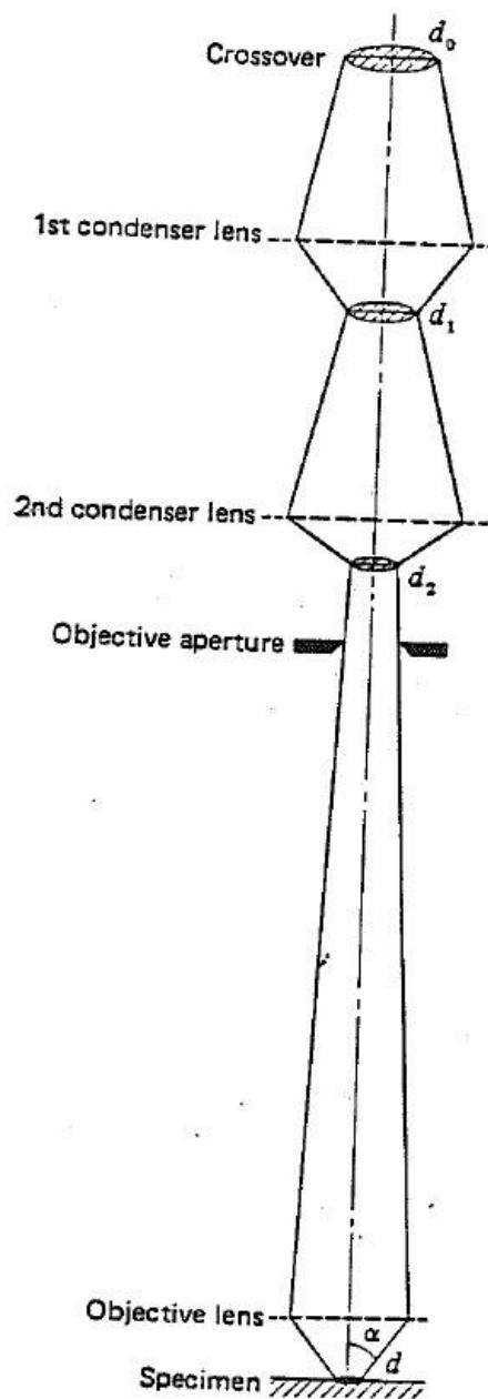
a configuration of the double condenser lens and objective lens in a SEM....
