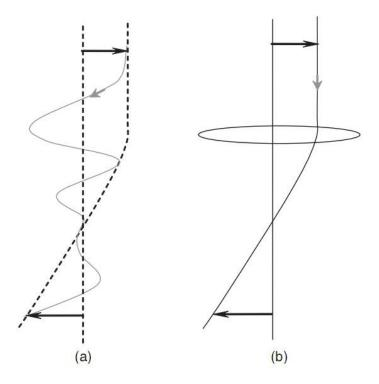
(a) Diagram showing how electrons passing through an electromagnetic lens are brought to focus; (b) a conventional optical ray diagram for comparison. Electrons rotate along this path (rotation omitted for clarity). Notice how the envelope marked by the dashed line in (a) resembles that of the ray in (b)
