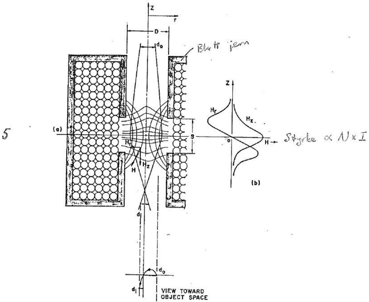
a cross-sectional view of an electromagnetic lens with the detailed magnetic field distributions, at any point of the pole-piece, a "composite" magnetic field could be divided as  $H(r)$  and  $H(z)$ ....
