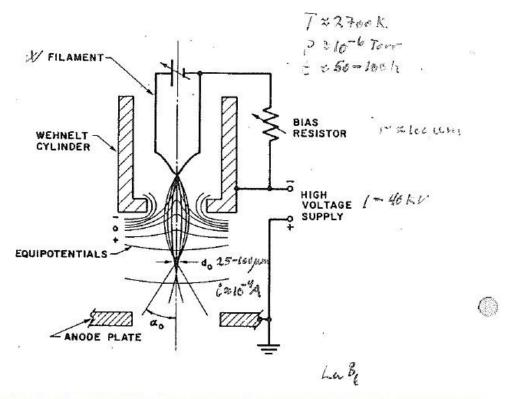
a negative potential applied to Wehnelt cylinder, together with an anode (connected to ground potential) to limit electron emission only from filament tip (for better coherency) down to first crossover ... GUN BIAS-current passed through the filament ("heat up" to get thermal emission)....
