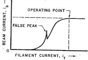
there is always a so called "saturation point" for a thermal emission gun, to further increasing filament current beyond saturation point, there is no any further benefit than decreasing filament lifetime....
