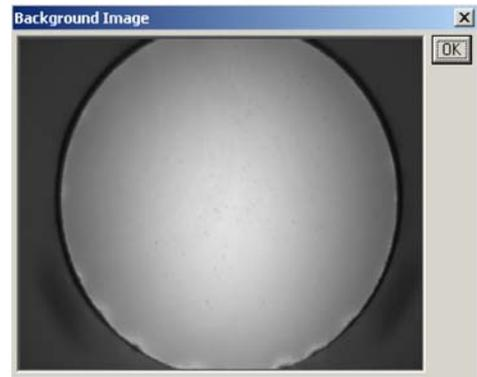
It should be noticed the beam illumination conditions etc. during the background calibration should be similar as that used during the later EBSD mapping. Also it is very important to notice, there is no visible EBSD pattern appeared on the background image during calibration. However it is very hard to avoid for some fine crystalline specimens, such as Si wafer etc. In such cases, the SEM should be setup at the fast TV scan mode, together with a relative lower SEM magnification.
