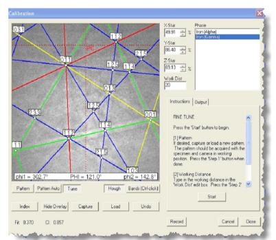
EBSD indexing by using  $\gamma$ -Fe (Cubic, m3m, a = 0.365 nm)
