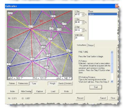
EBSD indexing by using Si (Cubic, m3m, a = 0.543 nm)
